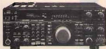
KENWOOD TS 850 S/AT RTX in SSB, CW, AM, FM e FSR - 100 kHz a 30 MHz - 108 dB - 100 W - 100 memorie - presa RS 232 - 2 VFO.
